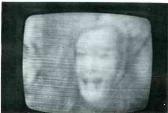
Fig. 7 Arcs across R340 shown in Figure 6 caused these horizontal streaks.
