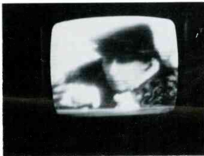
Fig. 5 Horizontal bands where the focus is different were caused by a defective focus-rectifier diode, SE1 in Figure 4.
