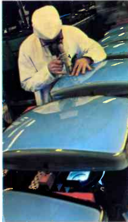
Microscopic inspection for precise placement of phosphor dots takes place in a GE clean room.
