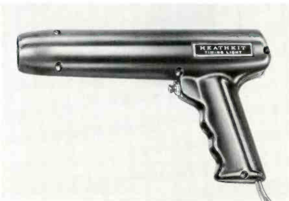
Fig. 3 Details of the Heathkit Timing Light. (left) In appearance, the timing light resembles an automatic pistol. Inside are a transistorized power supply, flash tube and a lens system. (right) Q1 is an audio oscillator supplying AC for rectification. DC is stored in C3 ready for use by the flash tube when it is triggered by a pulse from the spark plug.
