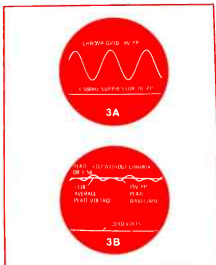
Fig. 3 DC plate voltage measured +112 volts without either chroma or carrier signals, and +118 volts with strong chroma but no carrier. Under these conditions, the demodulator is positive-going and is the reason for all-green color bars in actual receivers.
