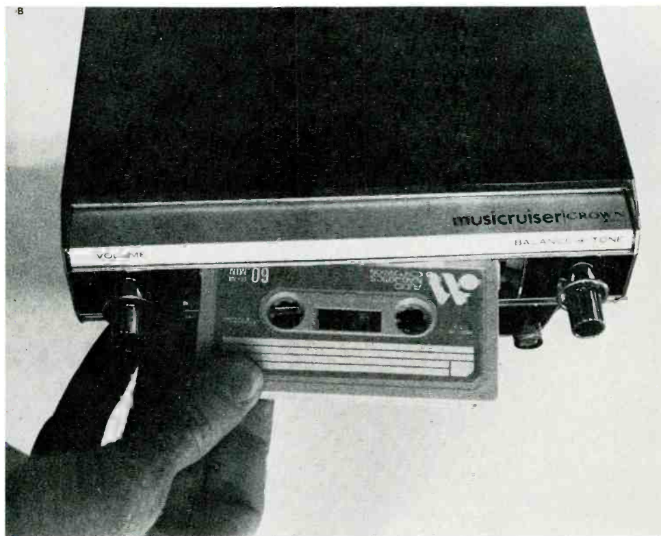
Fig. 1 Ordinarily, cassette loads (A) from top. Star system (B) permits slot loading; makes auto cassette machine feasible.
