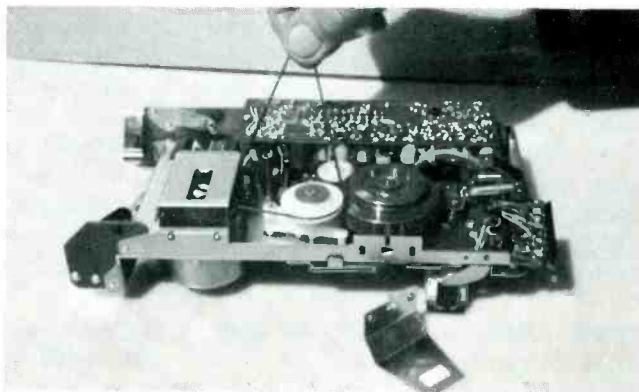
Fig. 14 Bearing bracket removed to permit belt replacement.
