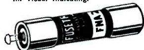
FNA FUSETRON Fuse 13/32 x \frac{1}{2} in. slow-blowing, Visual-Indicating, Alarm-Activating. (Also useful for protection of small motors, solenoids, transformers in machine tool industry.)
