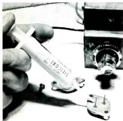
Fig. 7. Applying silicone grease to power output transistor.
