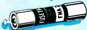
FNA FUSETRON Fuse 13/32 x 1 \frac{1}{2} in. slow-blowing, Visual-Indicating, Alarm-Activating. (Also useful for small motors, solenoids, transformers in machine tool industry.)
