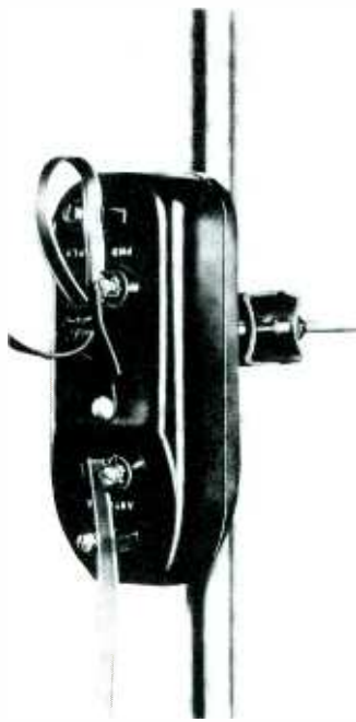
Fig. 3. Mast-mounted TV amplifier.
