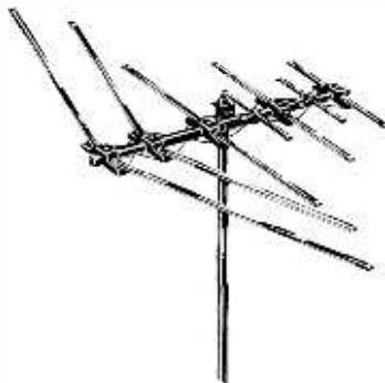
Fig. 10. Typical all-channel antenna.
