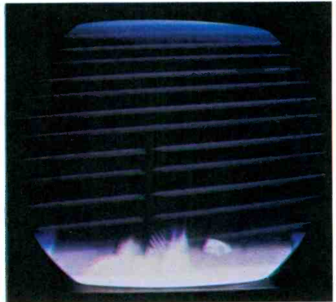
Fig. 3. Black raster, heavy, retrace lines due to H-K short.
