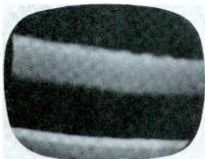
Fig. 9. Open C1 in full-wave circuit produced this raster.
