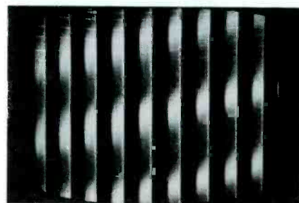
Fig. 2. Keyed-rainbow pattern with a small color sync error.
