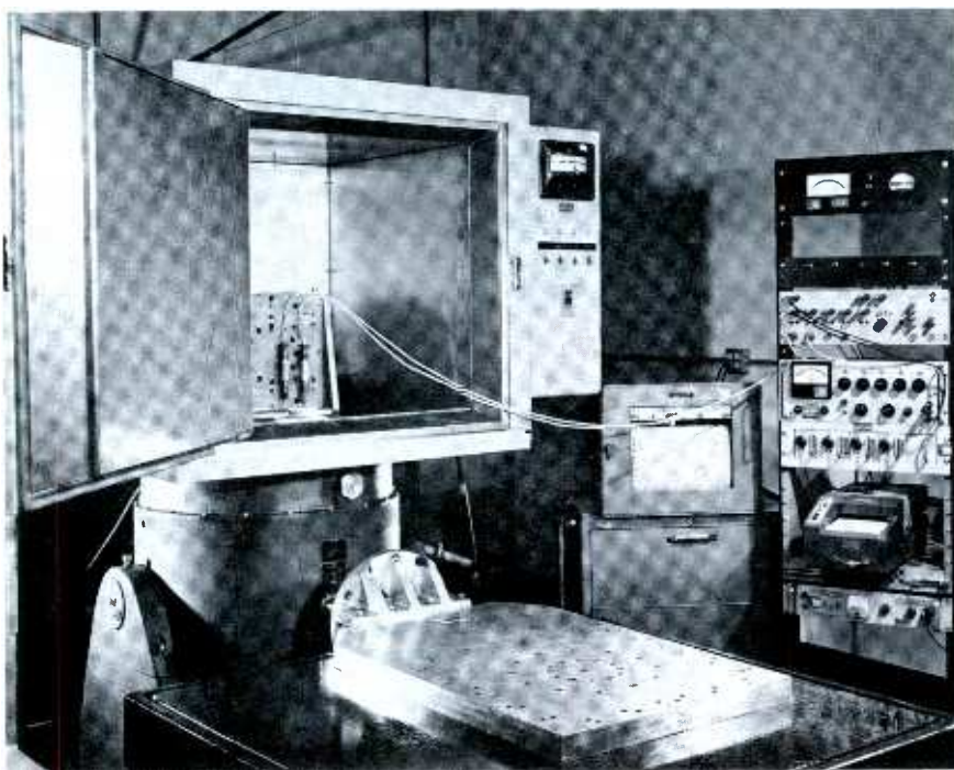
Fig. 1. Shaker attached through floor of temperature chamber.
