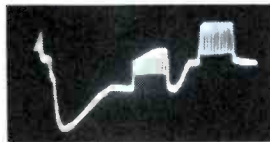
Good duplication of station signal including back porch. If the set won't sync, the set is defective.
