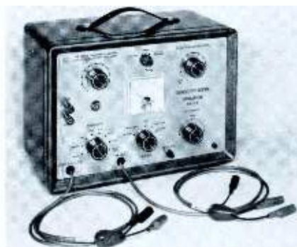
Fig. 1. Shows the new RCA Model WR-52A stereo-FM generator.
