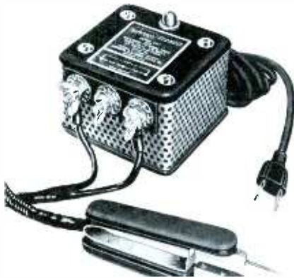
Fig. 7. Resistance-soldering unit provides high temperature in small area.
