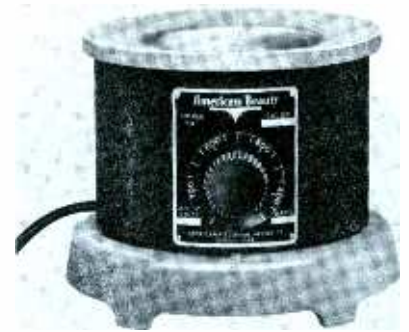
Fig. 8. Parts are fluxed then dipped in pot. Solder adheres to fluxed area.
