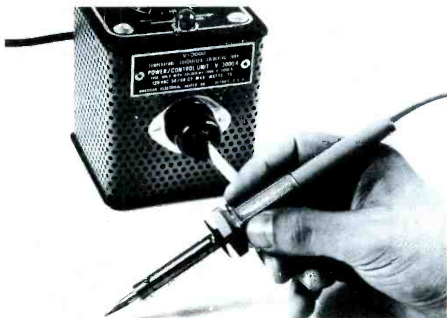
Fig. 5. Soldering iron uses sensor for temperature control.
