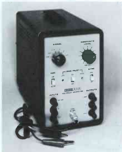
Fig. 1. This generator has many signals for multiplex testing and alignment.
