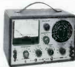
New Model 965 — FaradOhm Bridge/Analyzer. 9-range, low-voltage capacitance-resistance bridge safely measures even 1-volt electrolytics. Metered bridge balance, leakage test voltage (6 DC VTVM ranges 1.5-500V), leakage current (11 DC VTAM ranges 0.15ua-15ma). DC VTVM & VTAM externally usable. $129.95 wired.
