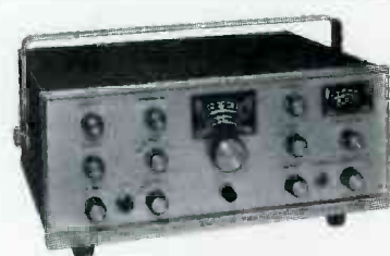
New Model 753 — The one and only SSB/AM/CW Tri-Band Transceiver Kit. 200 watts PEP on 80, 40 and 20 meters. Receiver offset tuning, built-in VOX, high level dynamic ALC. Unequaled performance, features and appearance. Sensationally priced at $179.95 kit, $299.95 wired.
