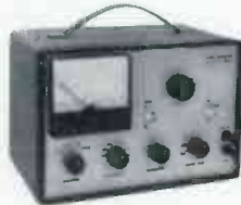
New Model 378 Audio Generator. Near-distortionless sine wave generator (< 0.1% 20-20,000c) providing fast, convenient, switch-selection of frequencies from 1c to 1,000c (1c steps 10c-100c, 10c steps 100c-1kc, 100c steps 1kc-10kc, 1kc steps 10kc-100kc). 8-pos. 10db/step output attenuator & fine attenuator. Output meter (4 1/2" 200ua) with 8 voltage ranges & db scale. $49.95 kit, $69.95 wired.
