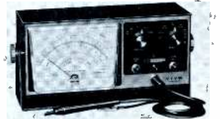
Fig. 3. Gimbal mounting of this VTVM allows adjustment for easy viewing.
