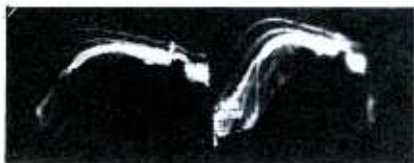
Fig. 5. Interstage screen-voltage connection causes this unusual symptom.
