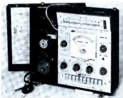
Fig. 1. CRT tester has compartment for cables and the adapter sockets.
