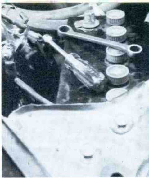
Now, under the hood, remove the battery ground cable while you fasten the hot wire of the receiver to the starter switch.
