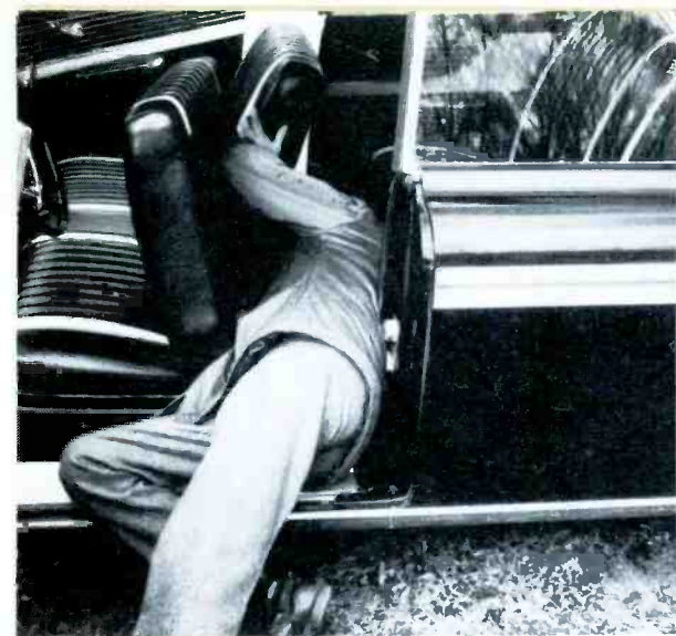
The lead-in cable goes under the floor mats. Push the plug end forward and the other end under the rear mat and seat.
