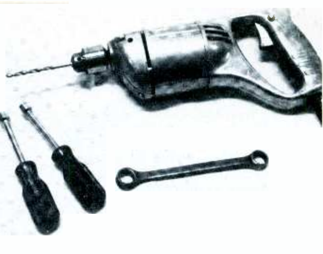
The installation doesn't require any special tools. You'll need a 1/2" box-end wrench, a couple of "spintites," 3/8" and 11/32", and possibly the few others that are shown here.
