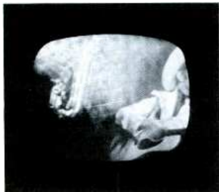
Fig. 2. Herringbone from RF signal.
