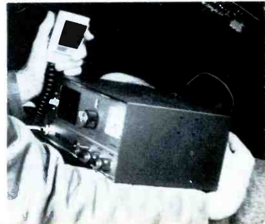
The receiver may be mounted under the center of the dash, or on the right side, or even on top—a handy position for pickup trucks. The top mount is accomplished by using two pieces of aluminum "angle" bolted to the sides of the case, with a third piece between them. Place a rubber pad over this third bracket. Lastly, follow instructions and tune up the transmitter.
