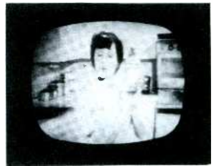
Fig. 9. Motor noise causes pix streaks.
