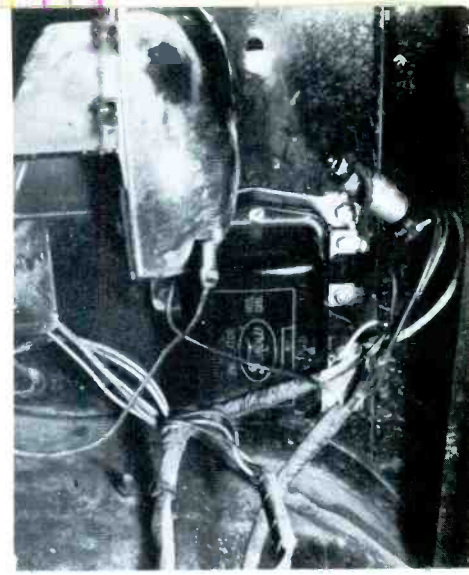
For best reception, install bypass capacitors on the generator armature and voltage regulator; coaxial types are best.
