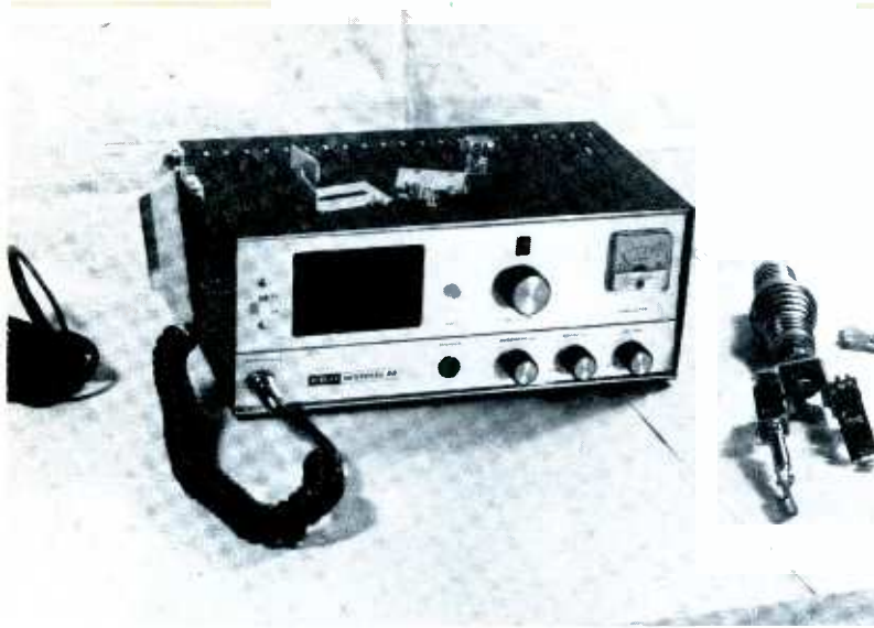
Here we see the equipment that must be installed: power and lead-in cables, antenna, and receiver. The most logical procedure is to install antenna, cables, and set, in that order.
