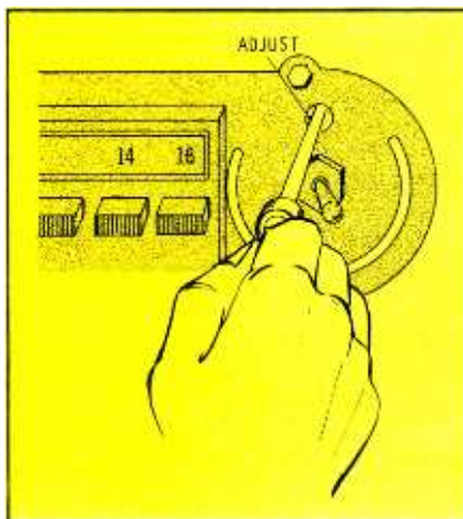
Fig. 1. Correct adjustment of antenna trimmer will improve reception.
