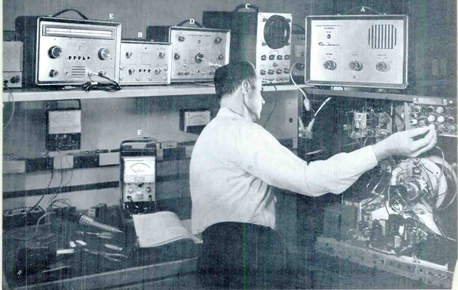
Making last-minute convergence adjustments on a color-TV receiver with an RCA WR-64A Color-Bar/Dot/Crosshatch Generator.
