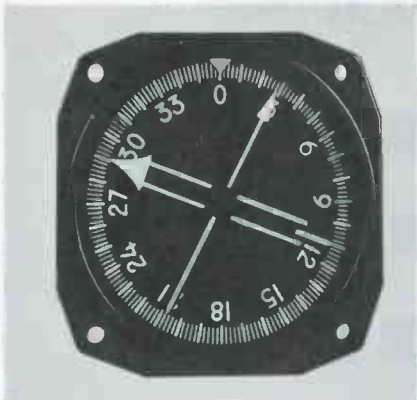
Fig. 6. Radio magnetic indicator gives all information on a single meter.
