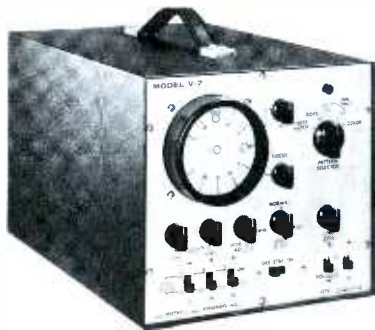
Fig. 9. Instrument combining a color generator and a color-vector display.
