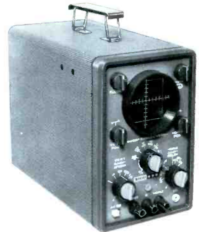
Fig. 8. Compact wideband scope is intended for servicing color or B & W TV.
