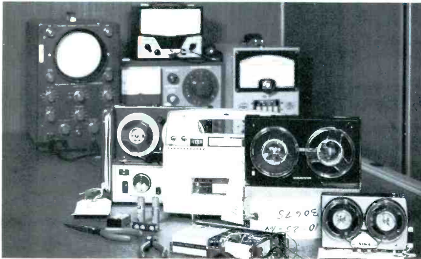
Fig. 8. Compact wideband scope is intended for servicing color or B & W TV.
