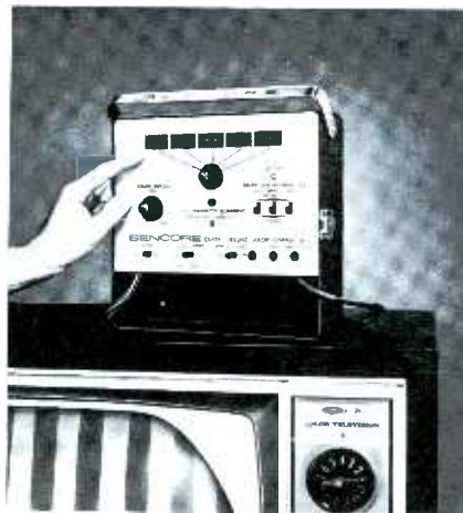
Fig. 5. Color generator features solid-state design, individual gun killers.
