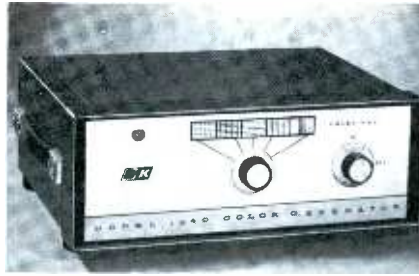
Fig. 3. Generator provides 5 patterns; gun killer is available as accessory.
