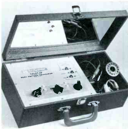
Fig. 7. Dot and line generator is synchronized from receiver yoke winding.
