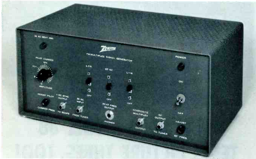
Fig. 1. Simplified unit offers complete FM stereo alignment with only one audio tone.
