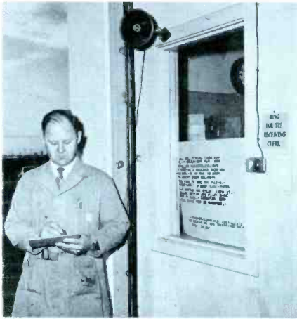
Extension loudspeaker at base station permits more flexibility of personnel in charge.
