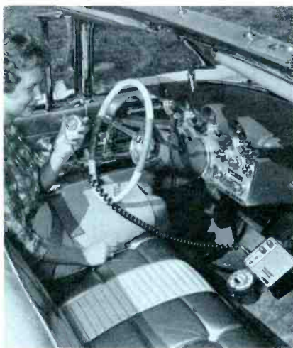
Dial used with class A Citizens band radio lets driver dial desired station or number.
