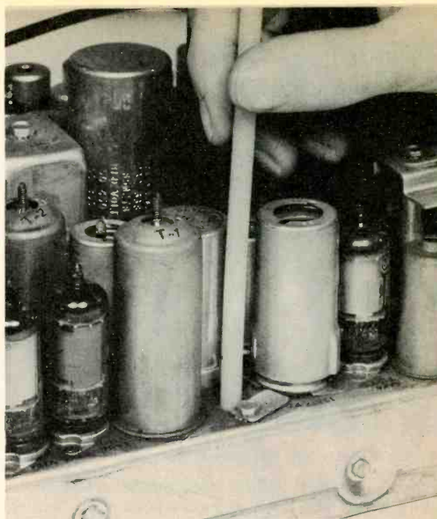
Fig. 7. The modulation control is usually beneath the chassis.
