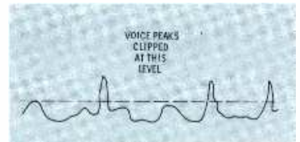
Fig. 1. Most effective power is below line.
