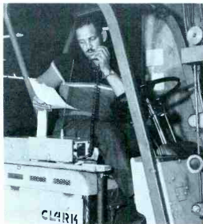
Metal box contains resistors to drop voltage to 12 volts on electrically-propelled vehicle.
