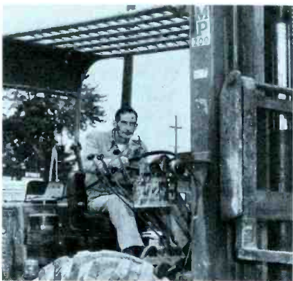
Both class A and D are used on material vehicles. Unit here is class A (460-470 mc).
