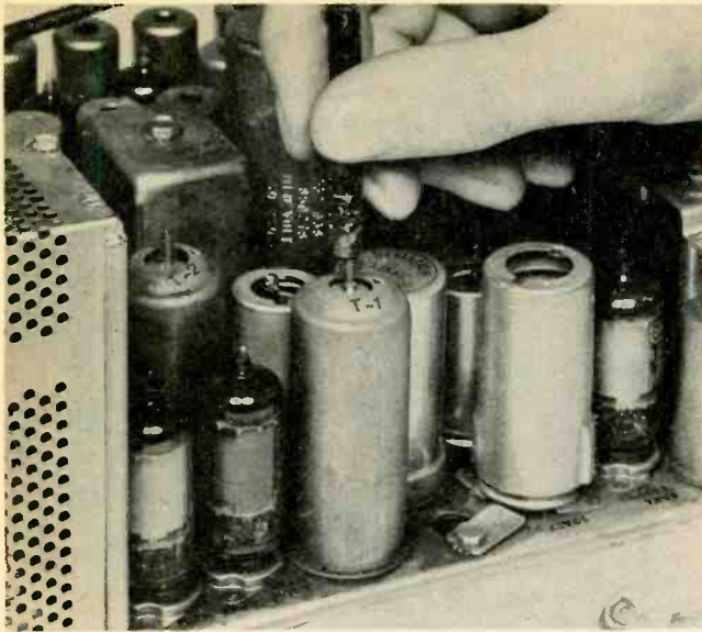
Fig. 9. Multiplier coils are aligned for a peak VTVM reading.
