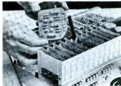
Fig. 2. Modular construction is sometimes used in transistorized preamps.
