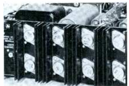
Fig. 9. Eight output transistors of 100-watt amplifier require heat sinks.
