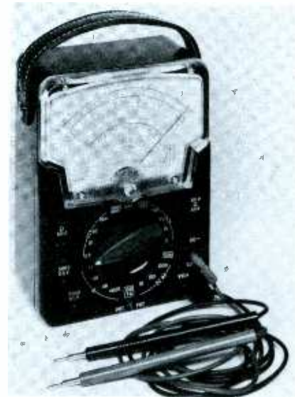
Fig. 1. Triplett 630-L has low-current ranges for transistor servicing.
