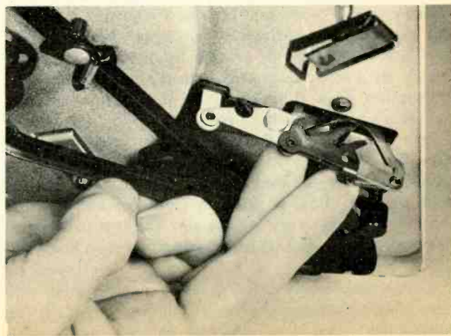
Fig. 14. Plate with notches controls setdown position of arm.
