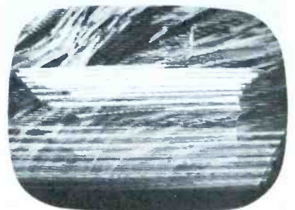
Fig. 11. Squegging caused by fault in operation of a triode-type AFC stage.
