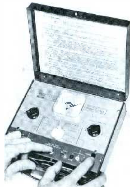
Fig. 3. Setting one switch and pressing pushbutton make up testing procedure.
