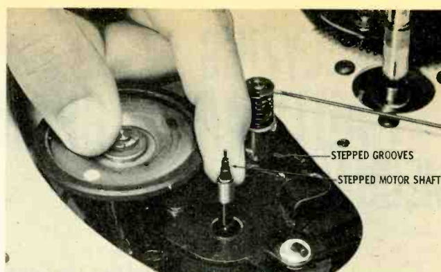
Fig. 3. Stepped motor shaft for changing speeds. Note idler plate raised and lowered by moving over stepped grooves.
