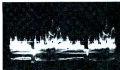
(B) Possible result of misaligned IF Fig. 2. Distortion of detected video.
