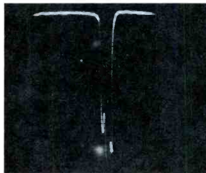
(C) AFC pin 7 (over 200V p-p) Fig. 9. Abnormal traces in first set.
