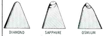
Fig. 4. Playing 15 LP records caused this much wear on different needles.
