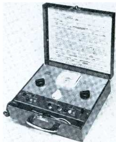
Fig. 1. Compact transistor-testing instrument is contained in metal case.
