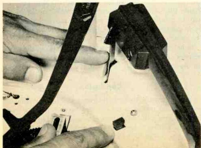
Fig. 13. Indexing sensors for both 10" and 12" record sizes.
