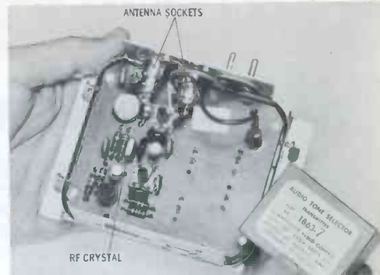
Fig. 3. Audio tone-selector circuit is enclosed plug-in unit in this set.
