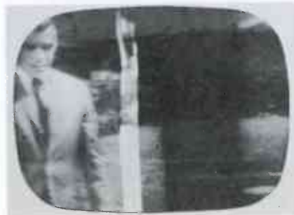
Fig. 6. Out-of-phase horizontal sync caused by faulty selenium dual diodes.
