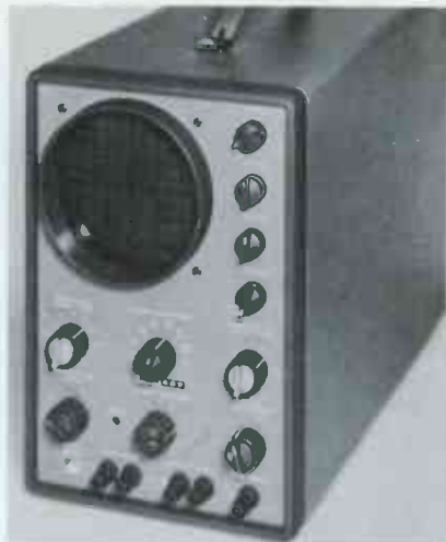
Fig. 4. This scope can be used for either AC or DC circuit measurement.
