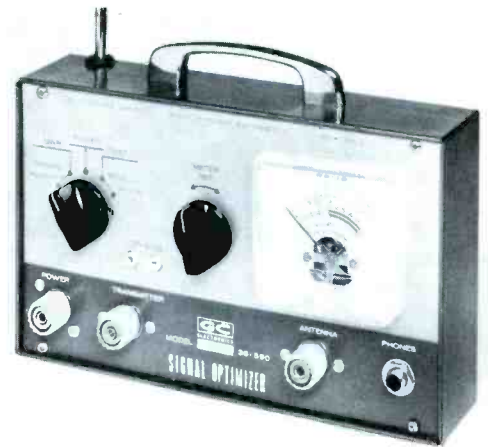
Fig. 4. Test unit has many purposes for servicing CB and communications units.
