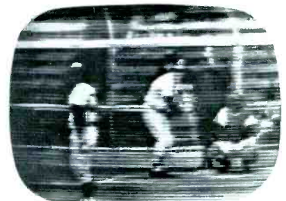
Fig. 8. Unusual variation on "Venetian blinds" due to bad AGC filter.
