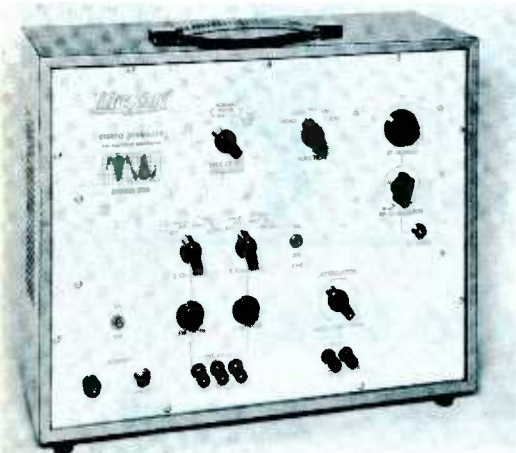
Fig. 1. New unit contains all signals needed for aligning stereo adapters.
