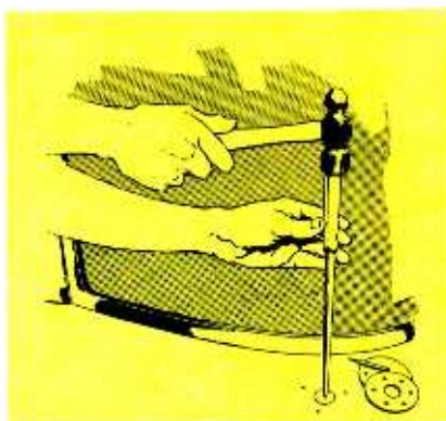
Fig. 2. Punch is used to mark center of mounting hole outlined in grease pencil.
