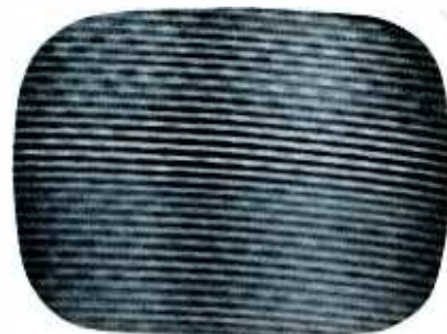
Fig. 11. Narrow horizontal stripes produced by oscillation in RF amplifier.
