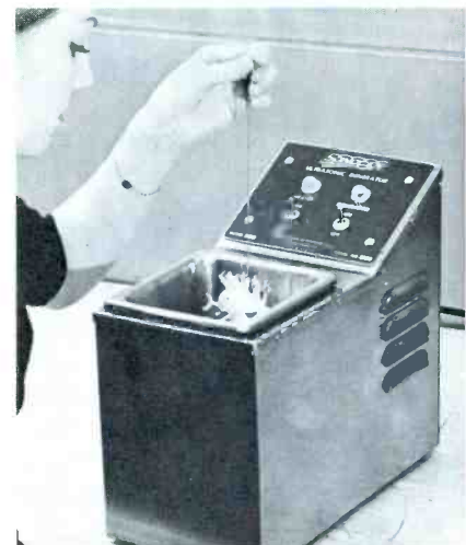
Fig. 3. Sonogen laboratory-type ultrasonic unit used to clean small parts.
