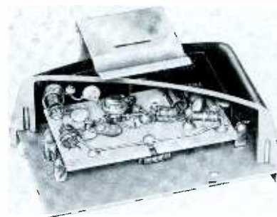
Fig. 13. Cutaway view of Winegard MA-300 showing internal construction.
