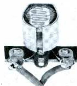
Fig. 3. Cadmium sulfide photoconductor changes resistance with light.
