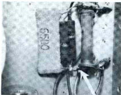
Fig. 11. Short between screen and filament resistors (arrow) was the culprit.
