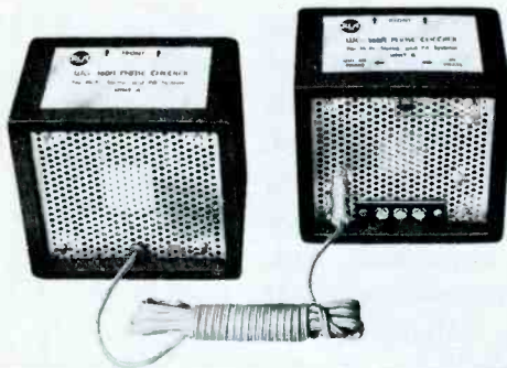
Fig. 1. Compact transducers help the serviceman check the phase of speakers.
