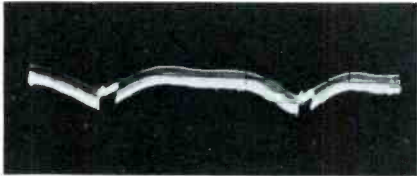
Fig. 11. Ripple on 150-volt B+ line (1.5V p-p) was the cause of distortion.
