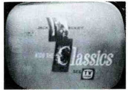
Fig. 4. In second case of horizontal bends, raster had billowed appearance.
