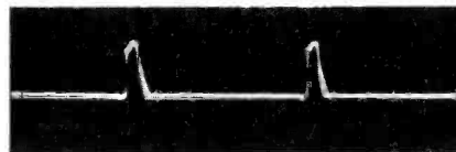
(A) Pulses only, indicating defect.
