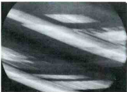
Fig. 12. Horizontal oscillator locked firmly in sync — on wrong frequency.
