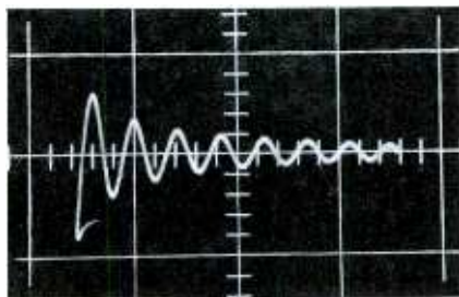
Fig. 5. Ringing test of bad yoke gave this overly-damped 120-kc waveform.
