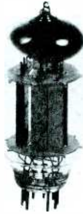
Fig. 3. New Sylvania 6EW7 vertical sweep tube has a standard 9-pin base.
