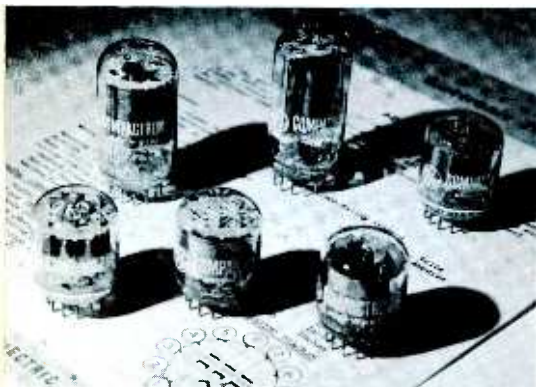
Fig. 1. G-E Compactrons. Left to right: 6C10, 6FJ7, 6B10, 6AX3, 6D10, 6K11.
