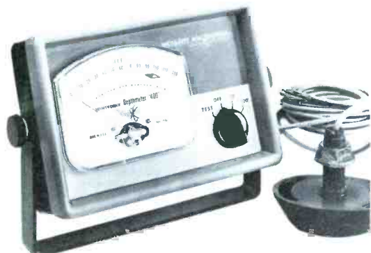
The Wintronix Depthmeter "400" is typical of direct reading units. A switch selects either of two ranges—one for depths up to 12', the other for depths to 120'.
