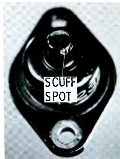
Fig. 1. The damaged spot on transistor case was evidence of a short to ground.
