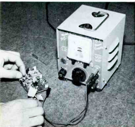
Fig. 1. PS-3 low-current DC supply offers automatic voltage regulation.
