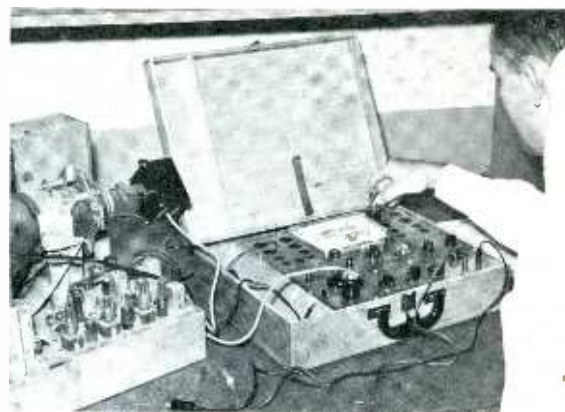
Fig. 4. A tube and capacitor checker, VOM, and CRT restorer all in one unit.
