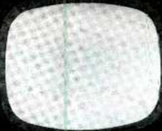
Fig. 2. Normal raster with antenna disconnected means "no regeneration."
