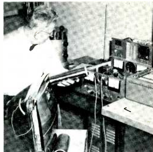
Fig. 5. Mr. W. H. Bradley, president of NMC, probes a tube for X radiation.
