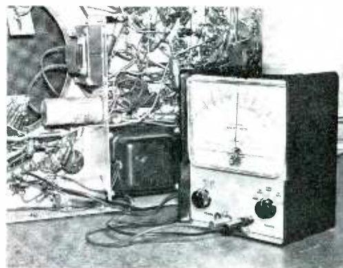
Fig. 1. Arkay's new meter measures capacitor values from 1 mmf to 1 mfd.
