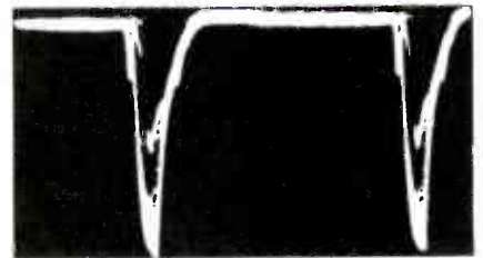
Fig. 9. Horizontal pulse amplitude fluctuates when 60-cps hum is present.
