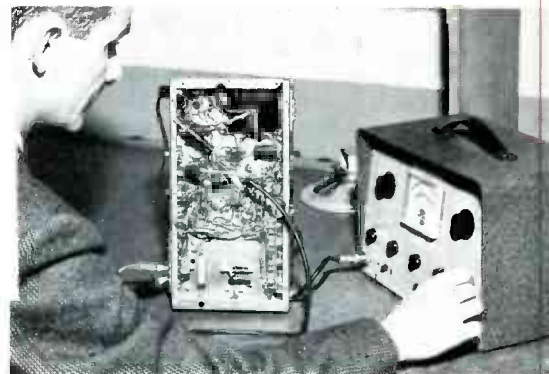
Fig. 7. Win-Tronix Analyzer is combination of audio-system test instruments.
