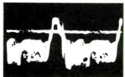
Fig. 3. Sync-input signal at 7875-cps sweep rate shows horizontal pulses.
