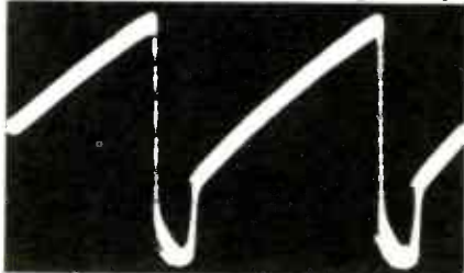
(C) Vertical drive signal.
