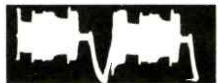
(A) Input to bandpass amplifier—mostly chrominance, some Y signal.
