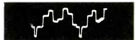
(C) Luminance or Y signal (composite video) at grid of video output tube.
