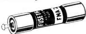
FNA FUSETRON Fuse 13/32 x 1 1/2 in. slow-blowing, Visual-Indicating, Alarm-Activating. (Also useful for protection of small motors, solenoids, transformers in machine tool industry.)
