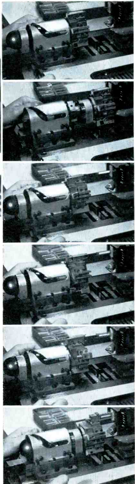
Large illustration shows operator completing the critical assembly work on a 6V6GTA mount in new CBS-Hytron automatic rotary assembly machine. Strip photos (top to bottom) catch six progressive steps: cathode positioned for insertion into bottom mica . . . cathode being inserted . . . A grid, B grid, and beam plate ready for assembly . . . top mica being added to complete the mount cage.
