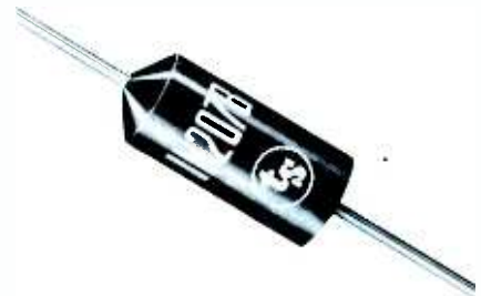
TUNG-SOL — Type 1N2078 pigtail style is designed for 100°C ambient temperature service. Ratings are: PIV 400 volts; DC output .625 amps; forward drop @ full load 1.1 volts; reverse current @ PIV .25 ma; minimum surge resistance 5 ohms.
