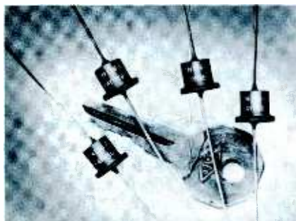
RAYTHEON — Types 1N1763 and 1N1764 are pigtail units with PIV 400 and 500 volt ratings respectively; DC output .5 amps; forward drop @ full load .9 volts; reverse current @ PIV .1 ma; recommended surge resistance 10 ohms.
