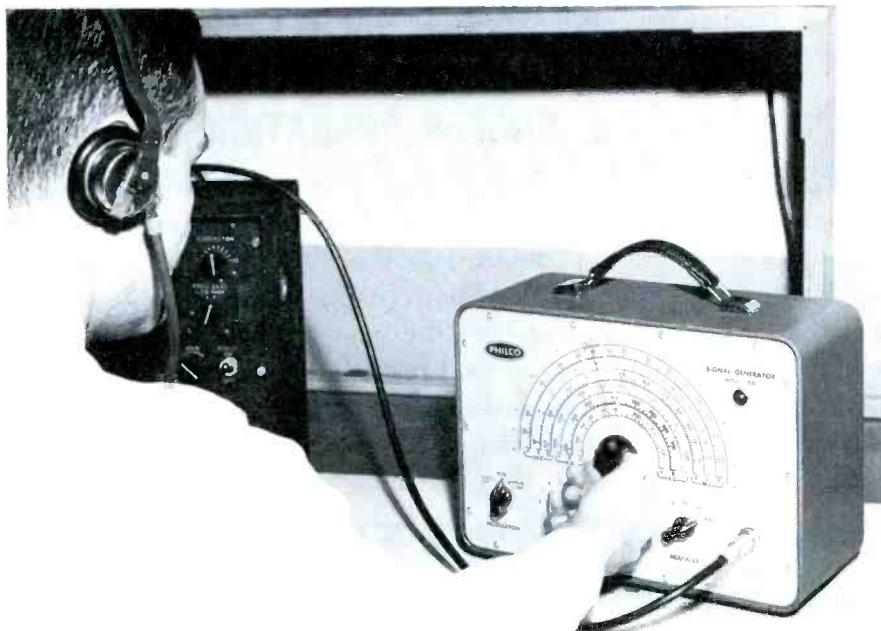
Fig. 1. Philco's RF generator is well-suited for radio and TV alignment work.
