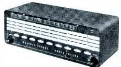
Fig. 1. Audio Baton has separate gain controls for nine different octaves.
