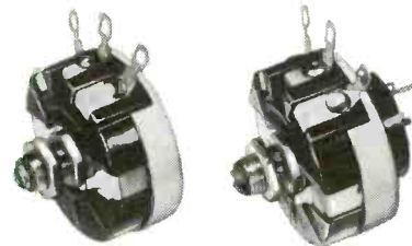
Series A 58: 3-watt wire-wound controls, 1 ohm to 50K ohms. Available with factory-attached switch, as Series A 58S (right).
