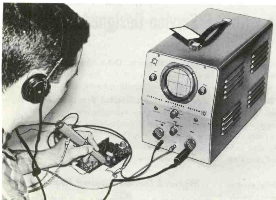
Fig. 4. Kingston Absorption Analyzer picks up signal radiation, converts it to standard IF frequency, and feeds it to high-gain scope for waveform analysis.
