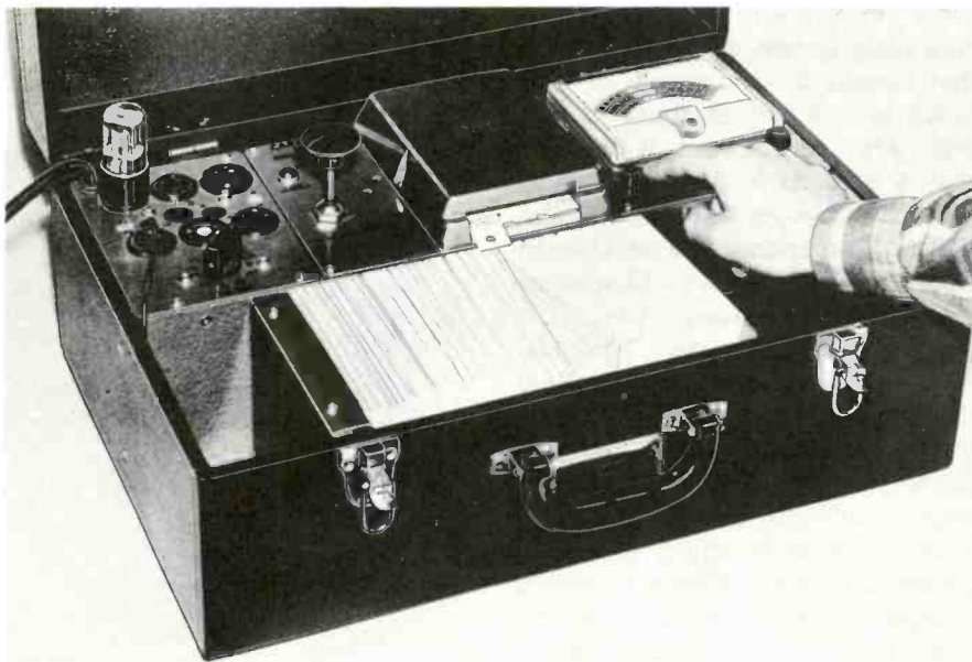
Fig. 6. Hickok Model 121 "Cardmatic" is a dynamic mutual conductance tube tester which uses prepunched, coded cards to set up conditions automatically.
