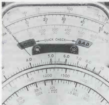
Fig. 6. Close-up view of the Model CRA-2 meter and resistance-capacitance scales.
