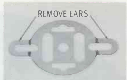
Fig. 2. Modified mounting plate required for installation of the new transformer.
