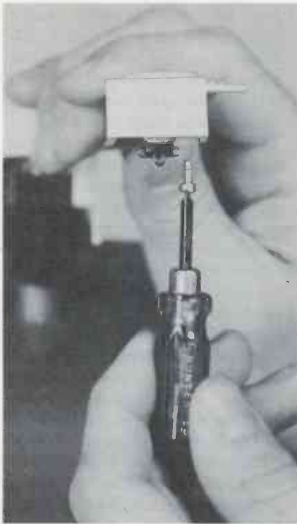
Fig. 3. Use of 2½" screwholding screw-driver speeds installation of cartridges.
