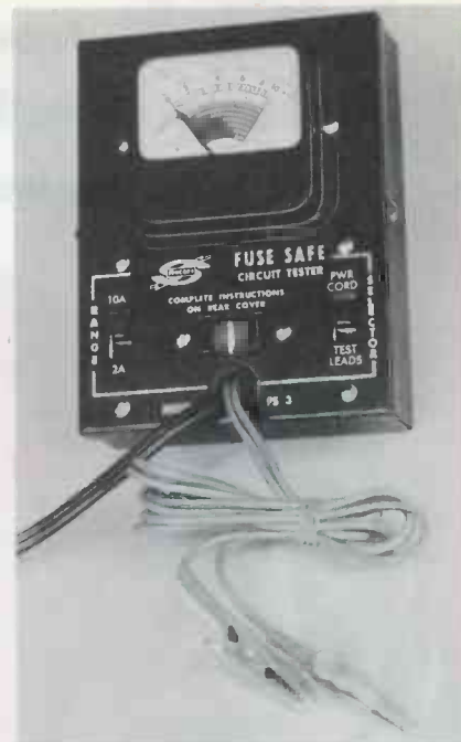
Fig. 4. "Sencore" Model FS-3 circuit tester is excellent for use on home calls.
