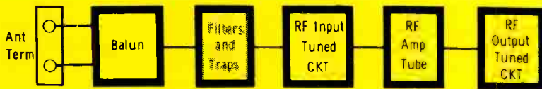
Fig. 1. Block diagram of the input and RF stages in a TV tuner.
