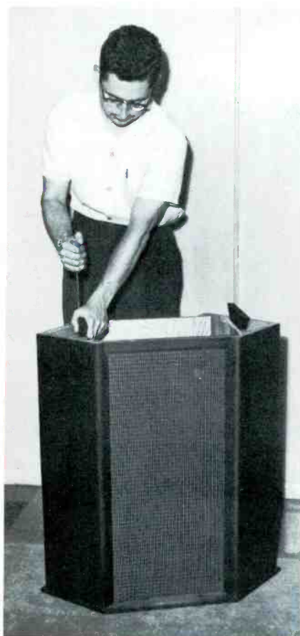
Fig. 1. This new RCA speaker enclosure is converted from an infinite baffle to a bass reflex cabinet by attaching legs.
