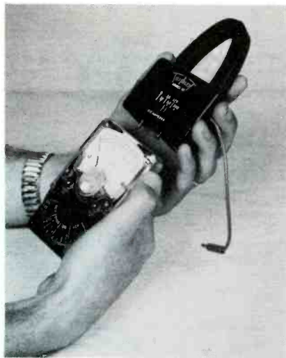
Fig. 6. New Triplet ammeter adapter fits right on pocket-size VOM.
