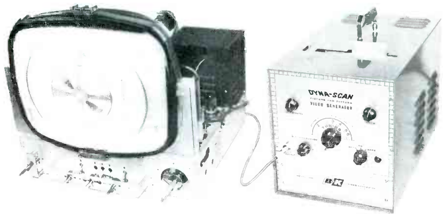
Fig. 1. B & K Model 1000 picture-pattern generator uses slide transparencies.
