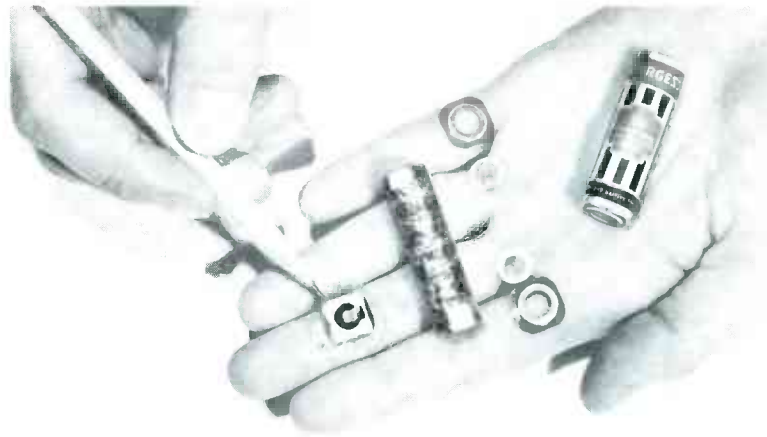
Fig. 4. Miniature 22½-volt battery contains a stack of cells individually sealed in transparent envelopes and bonded together with conductive wax.
