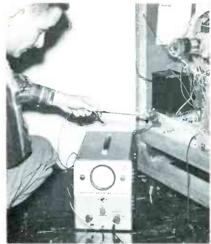
Fig. 4. Kingston Absorption Analyzer has a unique pick-up device.
