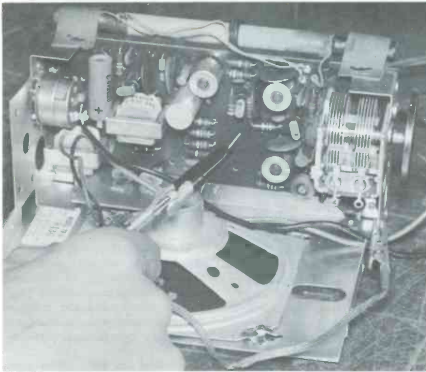
Fig. 5. A small tip on the end of the generator lead will minimize the danger of causing a damaging short.
