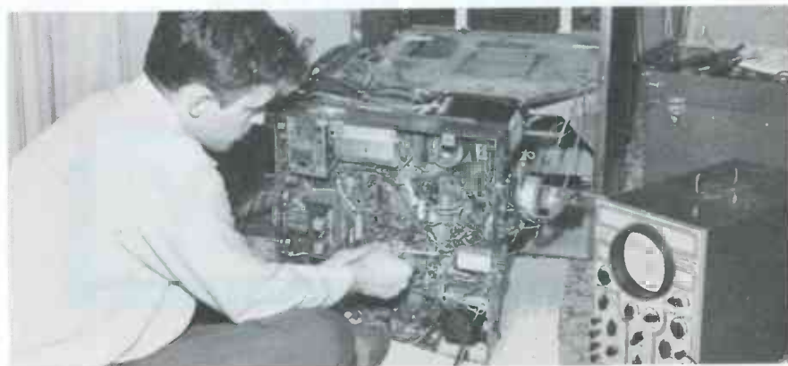
Fig. 4. Checking phase adjustment after slipping chassis out of cabinet.
