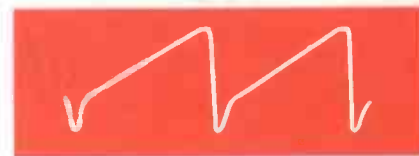
Fig. 3. Horizontal drive signal should have linear slope and minimum flat top.
