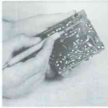
Fig. 3. In checking a printed board for shorted or broken conductors, an excess gob of solder may be located.
