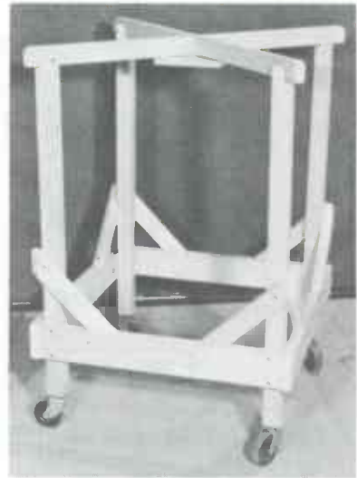
Fig. 1. TV test stand.
