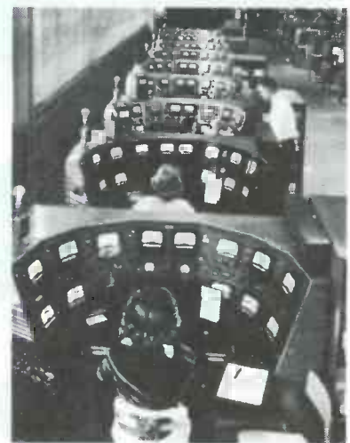
Dynamic TV set conditions are set up in these test bridges making the “fixed bias” test a true measure of how the tube will perform in TV sets encountered by you in the field.
