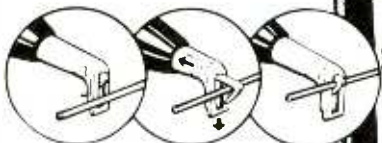
Place Foot Against Wire Push and Slide Release
