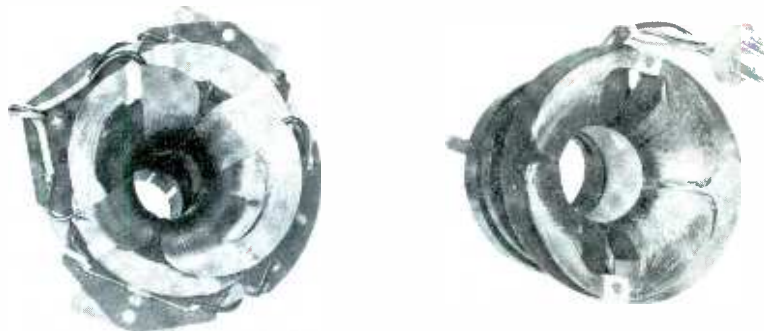
Fig. 2. Smaller center hole and severe flaring is shown by this comparison of the new 110°-deflection yoke (left) and a 90° yoke.
