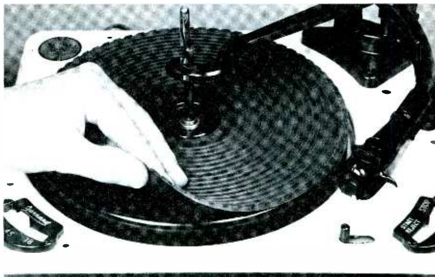
Fig. 5. A foam-rubber pad can be used to dampen vibrations. This will reduce rumble and also help prevent record damage.
