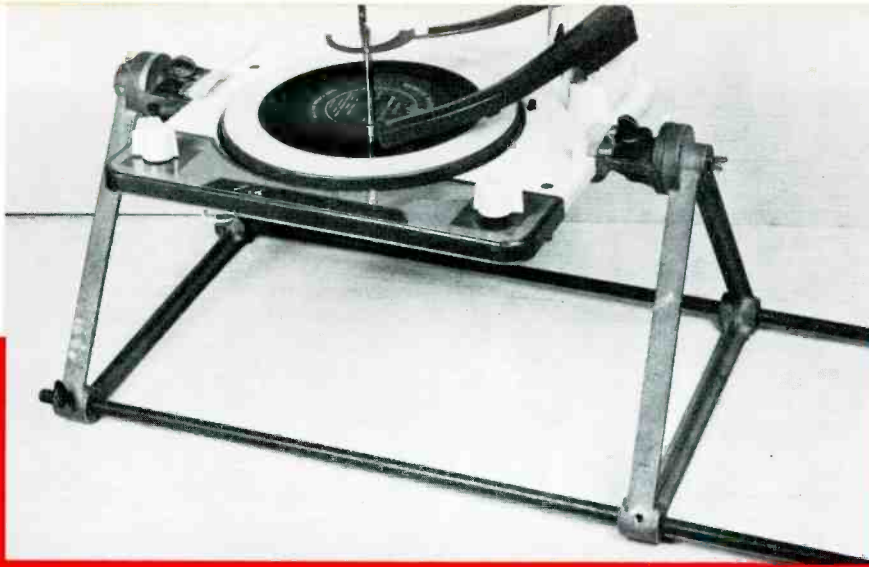
Fig. 1. A typical automatic record changer held in operating position by a handy support rack, a must in phono servicing.
