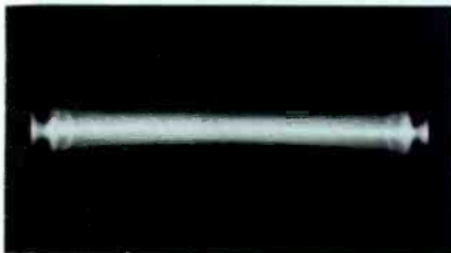
Fig. 11. Appearance of the Screen When the Vertical Sweep Has Failed.
