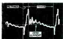
(C) Current Through the Transformer Winding. Fig. 4. Waveforms in the Circuit of Fig. 1.
