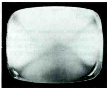
Fig. 4. Damaged Coating on the Picture-Tube Screen.
