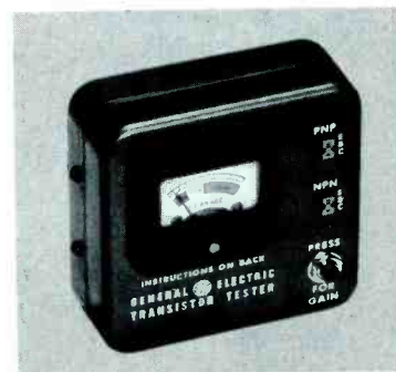
Fig. 4. The General Electric Transistor Tester. Its Circuit Is Essentially the Same As That Shown in Fig. 3.
