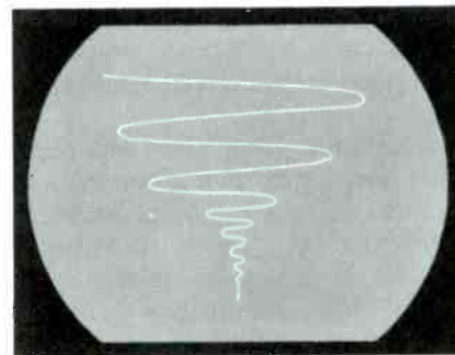
Fig. 10. Pattern Produced on the Screen As the Energy in the Resonant Loop Dissipates After the Damper Tube Fails or Is Removed.
