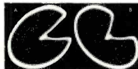
Fig. 20. Lissajous Patterns (A) With Quadrature Transformer Misadjusted in One Direction and (B) With Quadrature Transformer Misadjusted in Opposite Direction.
