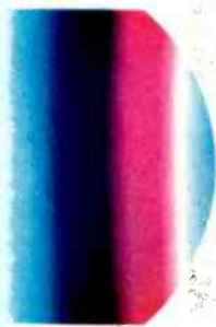
Fig. 14. A Plus I Signal Indicating Improper Setting of Hue Control.
