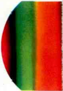
Fig. 10. Pattern Indicating Loss of Blue Signal.
