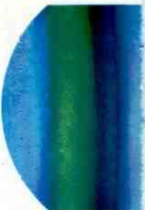
Fig. 8. Pattern Indicating Loss of Red Signal.
