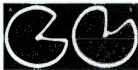
Fig. 19. Lissajous Patterns (A) With Hue Control and Quadrature Transformer Correctly Adjusted and (B) With Hue Control Incorrectly Adjusted.
