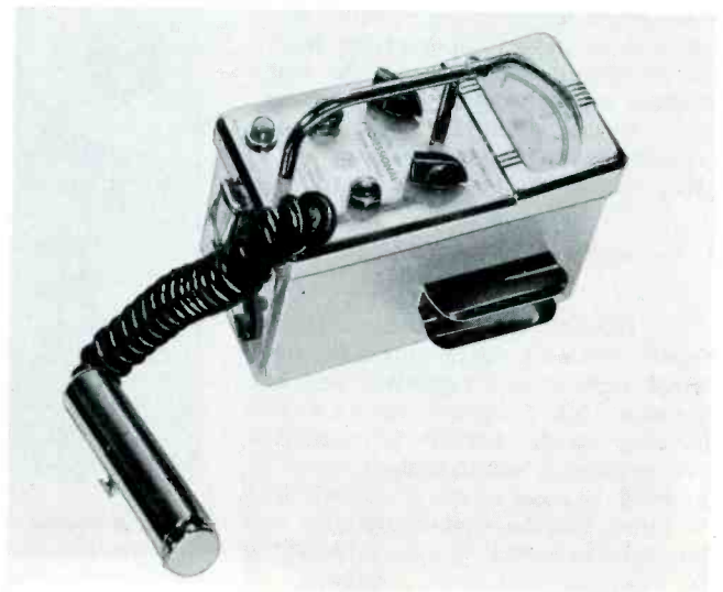
Fig. 1. Precision Model 107C Professional Geiger Counter.
