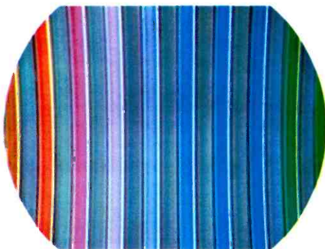
Fig. 3. Pattern Indicating Improper Setting of Hue Control.
