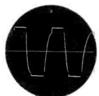
Mallory vibrator after hundreds of hours of service
