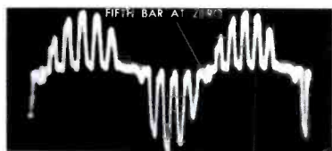
Fig. 14. Signal at Plate of I Demodulator Illustrates Proper Cancellation of Fifth-Bar Signal.
