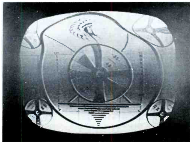
Fig. 7. Hum Bars Caused by 60-Cycle Modulation.
