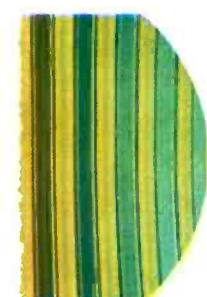
Fig. 14. Signal at Plate of I Demodulator Illustrates Proper Cancellation of Fifth-Bar Signal.
