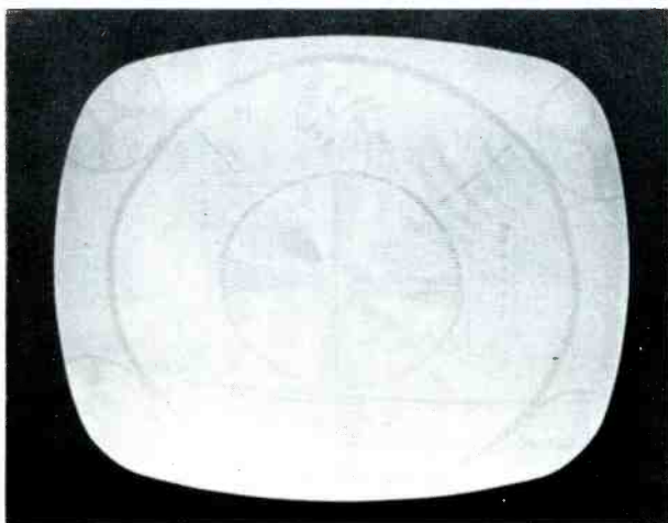
Fig. 3. Lack of Picture Contrast.
