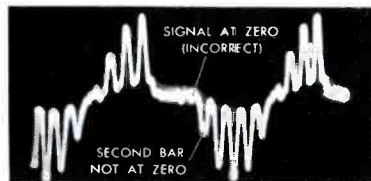
Fig. 17. Signal at Plate of Q Demodulator Illustrates Improper Cancellation of Second-Bar Signal.
