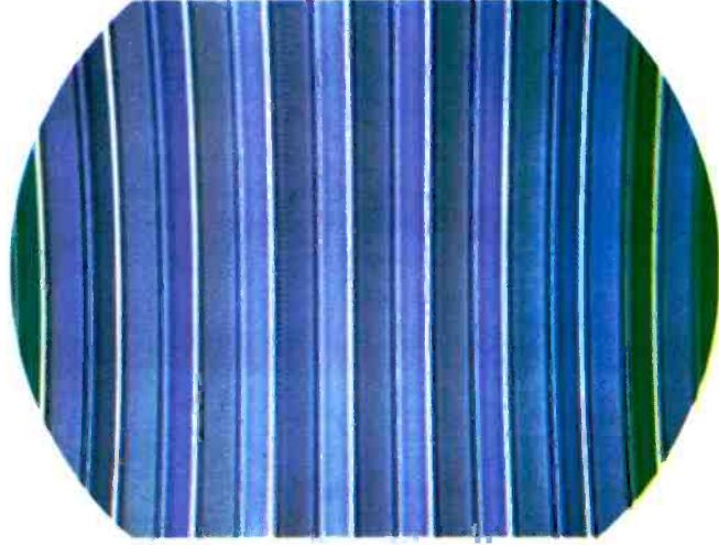
Fig. 6. Pattern Indicating Loss of I Signal.
