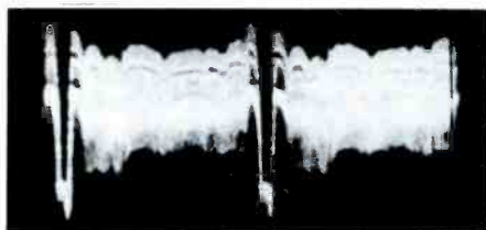
(C) Waveform Showing Sync Inversion.
