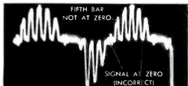
Fig. 15. Signal at Plate of I Demodulator Illustrates Improper Cancellation of Fifth-Bar Signal.
