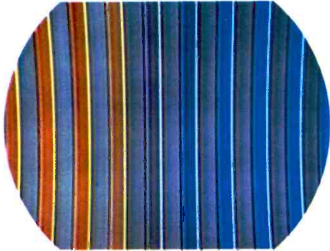
Fig. 5. Pattern Indicating Loss of Q Signal.
