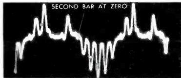
Fig. 16. Signal at Plate of Q Demodulator Illustrates Proper Cancellation of Second-Bar Signal.
