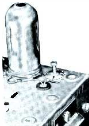
Fig. 2. Connection Into the Mixer Grid Circuit of the Tuner Can Be Made Easily Through the Projecting Loop Shown.
