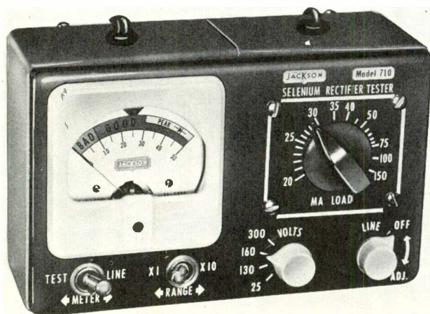
Figure 2. The Jackson Model 710 Selenium Rectifier Tester.
