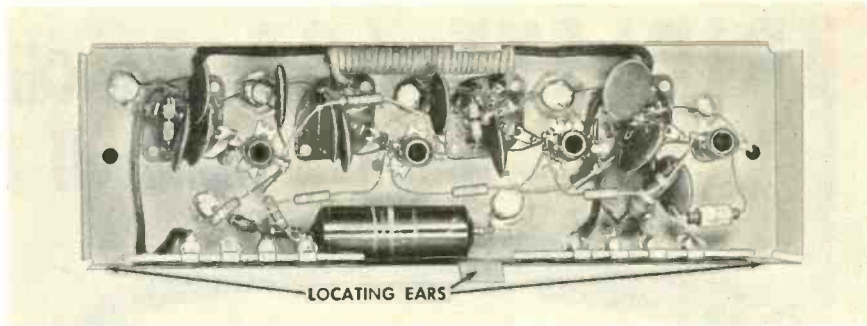
Figure 9. Video IF Sub-Assembly Unit in Setchell-Carlson Showing Terminal Jacks and Locating Ears.
