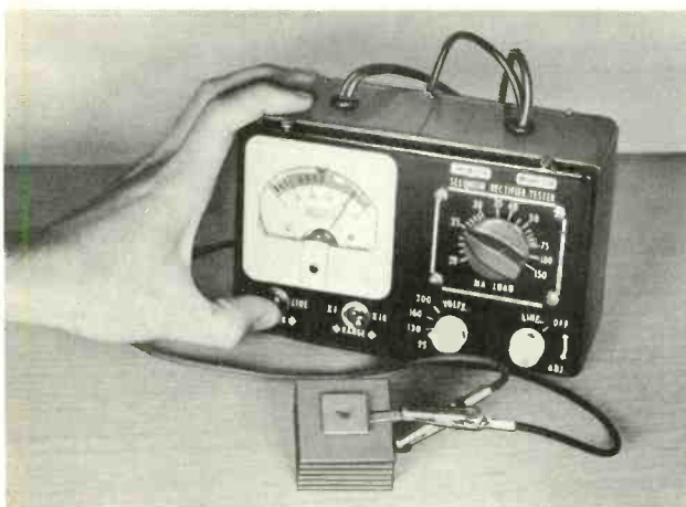
Figure 5. Test Setup of a Selenium Rectifier out of the Circuit.
