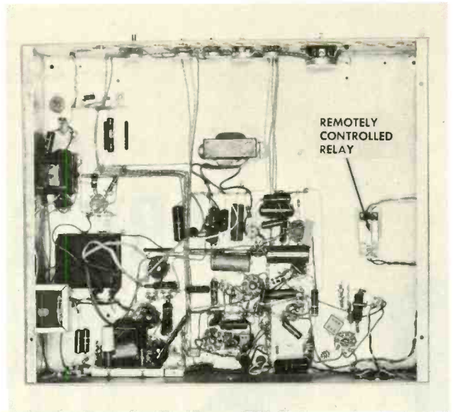
Figure 5. Bottom View of Sweep Chassis in Fleetwood 600 Receiver.
