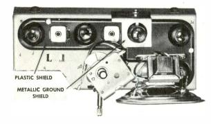
Figure 5. GE Chassis with Plastic Shield Surrounding Socket Terminals.
