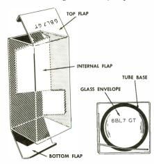
Figure 7. Diagram Showing Tube in Sylvania Tube Carton.
