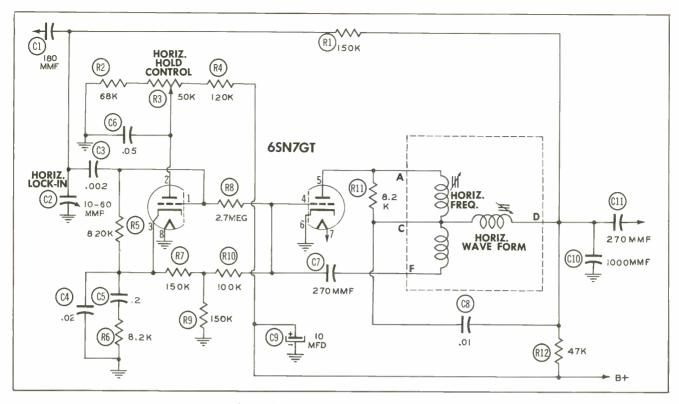
Figure 4. Typical "Synchroguide" Circuit.
