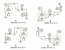
Figure 7-15. Charge and Discharge Paths of the Coupling Capacitors, C1 and C2 of Fig. 7-14.
