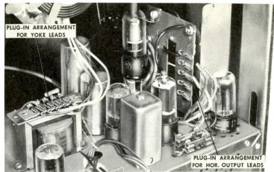
Figure 12. Plug-in Connections Employed on Horizontal Output Transformer and Deflection Yoke.
