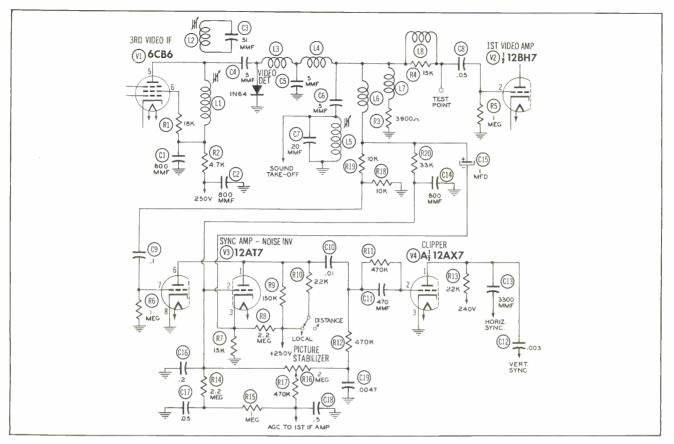
Figure 10. Partial Schematic of GE Model 21T1 Receiver.
