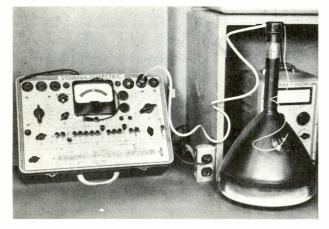
Figure 7. Sylvania Cathode Ray Tube Testing Adaptor Type 228.
