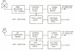
Figure 15. Block Diagram Showing Operation of KRK-12 Tuner.
