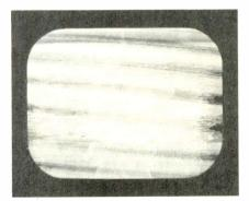
Figure 3. Random Operation of a Horizontal Oscillator Produces Characteristic "Christmas Tree" Effect.
