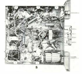
Figure 11. Stewart Warner Chassis Showing Component Grouping in 9300 Series (A) as Compared to 9200 Series (B).
