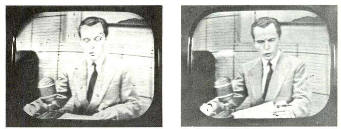
Figure 1. Picture Tube Having Low Cathode Emission. (A) "Zombie" Effect at High Brightness Setting. (B) Normal Shading at Reduced Brightness Setting. (Photographs Reproduced with Permission of CBS Television with Apologies to Winston Burdette.)
