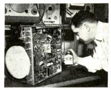
Because of its high dielectric strength, Krylon helps prevent corona. Here technician Bernard Vanella—on the staff of dealer Mort Farr, Philadelphia—"Krylon-izes" high voltage coil and insulation, the socket of the high voltage rectifier, component parts of the rectifier circuit.
