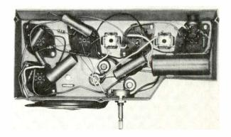
Figure 7. Bottom View of Model 542 Showing Completed Wiring.
