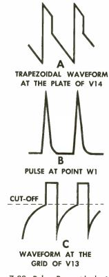
Figure 7-22. Pulses Present in the Wave Shaping Network of Fig. 7-21.
