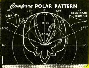
Model 848 Compound Diffraction Projector\* Loudspeaker System Conservatively rated at 25 watts. 16 ohms impedance. Finished in attractive gumetal gray. Two mounting positions for hang-up bracket. Projectors can be installed horizontally, or vertically for augmented dispersion. Dimensions: 10½" wide at mouth, 20½" high at mouth, 20" deep over-all. Weight: Net 12 Ibs., Shipping 15 Ibs. List Price...
