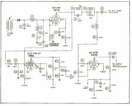
Figure 13. Partial Schematic of Video, Keyed AGC, and Gated Sync Separator Circuits.
