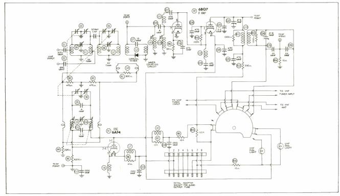
Figure 8. Schematic of Philco UHF Converter Model UT-21B.
