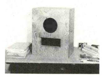
Figure 3. Front View of Reflex Enclosure Discussed in Text. Boards Used to Fill in Cabinet to Reduce Size Are Shown at Left.
