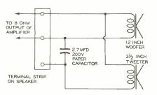
Figure 3. Schematic of Stromberg-Carlson RF-71 Speaker.
