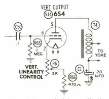
Figure 7-24. Vertical Output Circuit Employing a 6S4.
