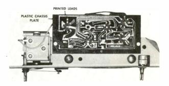
Figure 3. Printed Circuit Leads Formed on Plastic Chassis Plate.
