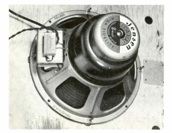
Figure 1. Jensen H-222 Coaxial Speaker with Capacitor Attached to Frame.
