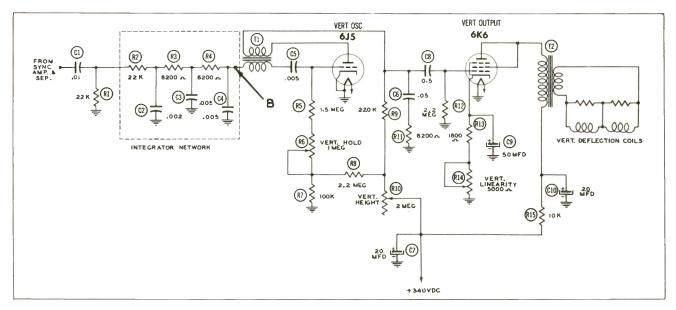
Figure 2. A Typical Vertical Deflection System
