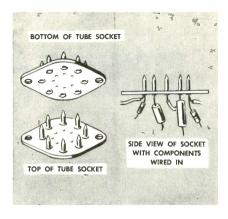
Figure 6. Construction Details of Socket Employing Hollow Tubular Terminals.
