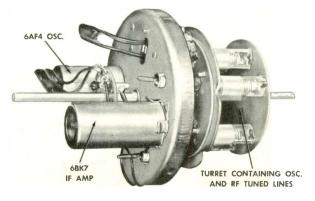
Figure 2. Photo of Tuner Turret with Shield Removed.
