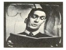
Figure 1. The Visual Effect Produced When 60-cycle AC (Hum) Enters the Video System.
