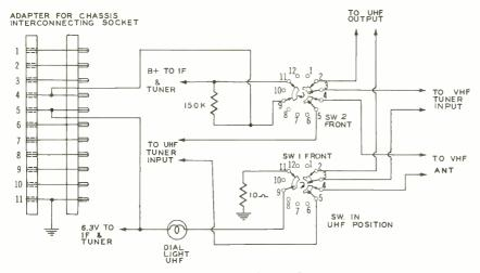
Figure 9. Function Switch and Adaptor for UHF Tuner UT-21.
