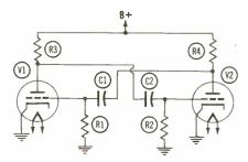
Figure 7-14. A Basic Multivibrator Circuit.
