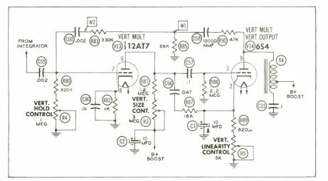
Figure 7-21. A Commercial Vertical Multivibrator Circuit Employing Two Triode Sections for the Multivibrator and Output Amplifier.
