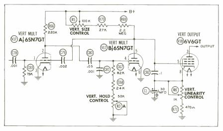
Figure 7-17. A Commercial Type Plate-coupled Multivibrator.
