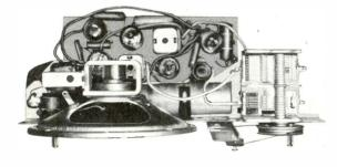
Figure 2. Component Arrangement in Admiral Radio.
