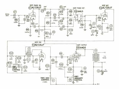
Figure 7-23. Vertical Sweep System Controlled by an AFC Circuit.
