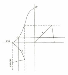
Figure 7-25. Removal of the Nonlinearity from the Sawtooth by Operating the Amplifier on the Curved Portion of the Characteristic Curve.
