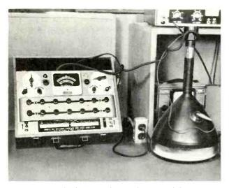
Figure 5. Cathode Ray Tube Analyzer Model 707 Produced by Jackson Electrical Instrument Co.
