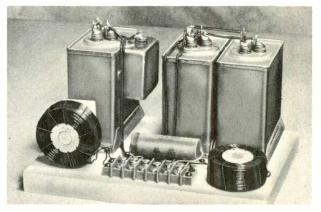
Figure 5. Home-Constructed Divider Network.
