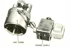
Figure 1. Photo of GE UHF Tuner Model UHF-103 with Included Power Supply.
