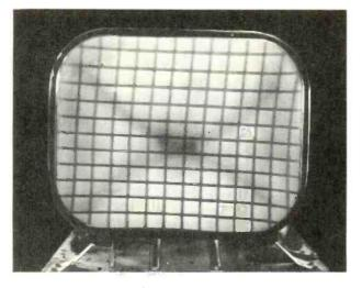
Figure 3. Severe X-shaped Ion Burn on a Rectangular 16TP4.
