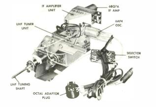
Figure 4. Philco UHF Converter Model UT-21A.
