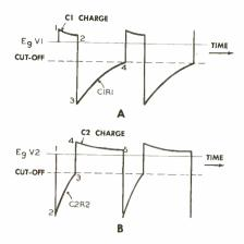
Figure 7-16. Grid Waveform of each Section of the Free-running Multivibrator of Fig. 7-14.
