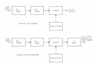
Figure 5. Block Diagram of Philco UHF Tuner and Converter.
