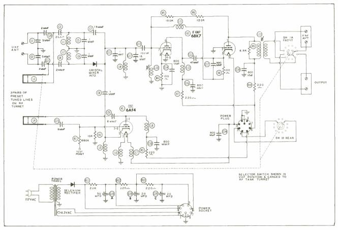
Figure 3. Schematic of GE Model UHF-103.
