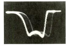
Figure 2. Response Curve with "Ghost" Produced by Horizontal Oscillator Radiation from TV Set.
