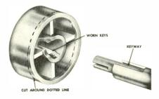
Figure 1. Worn Knob with Dotted Line Marking the Flange Cut.
