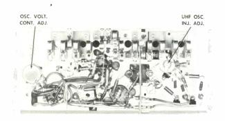
Figure 14. Under Chassis View of KRK-12 Tuner.
