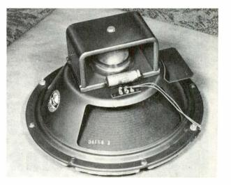
Figure 2. Stromberg-Carlson RF-71, Coaxial Speaker Showing Capacitor in Series with Tweeter.
