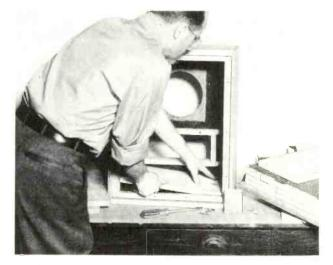
Figure o. Installing Boards to Reduce Cabinet Size.
