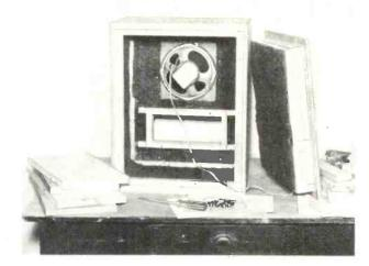
Figure 4. Interior View of Enclosure. Ozite Padding, Duct on Port and Boards Installed on Inside of Back to Reduce Cabinet Size Are Shown.
