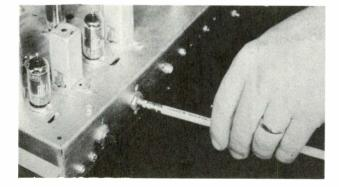
Figure 5. Using a Pencil as a Control Shaft Extension.
