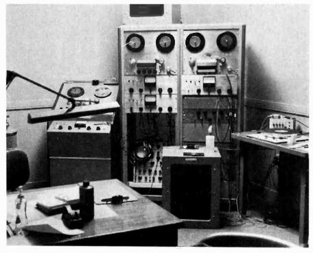
Modern recording facilities for duplicating tapes includes these twin Ampex professional tape decks, PSR Metrotec equalizers and other equipment.
