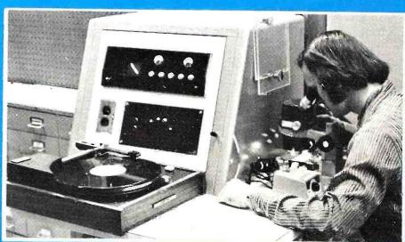
Turntable alignment system developed by Myer-EMCO.
