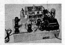
Innards of one of the better performing pre-war FM tuners, the G.E. JFM-90. This set tuned the 42 to 50 MHz band and boasted a sensitivity of 4 microvolts for 20dB quieting. This was considered very good in those days as most FM receivers claimed only 10 microvolts.
